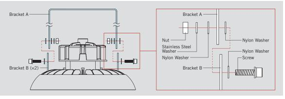
3. Adjust the angle of bracket A and then affix to each bracket B using mounting hardware provided.
