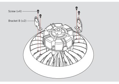
2. Attach bracket A to both brackets B using mounting hardware provided.
